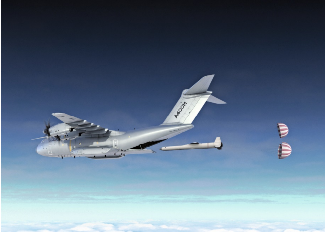
Fig. 1: Eject of a launcher over the tail ramp of a military transport aircraft.
